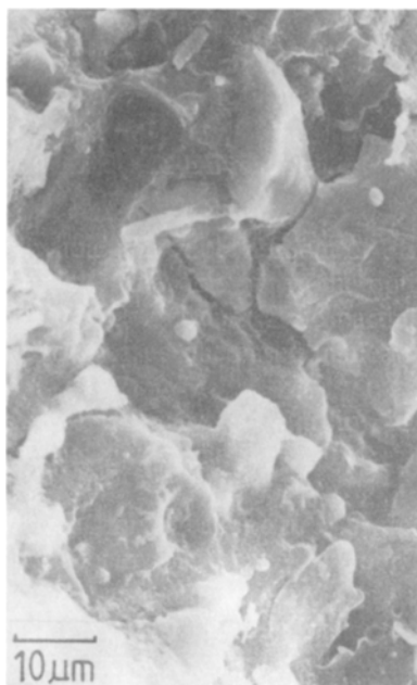
Fig. 3 SEM micrograph of 29% IFR containing PP sample after etching with heptane
